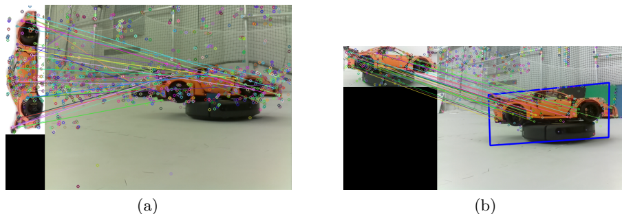
Fig. 3: (a) Example image matches between the reference object image (left) and an experimental image (right): Circles represent features, and lines indicate matches. (b) Homography and localization of car with prospective transform of bounding box.
